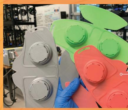
An early prototype of N95-modeled respirator masks is shown here. Heat was later applied to form the masks into a face-fitting shape
